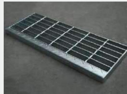
Welded fixing, banded ends with checker plate nosing.
